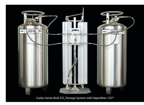
The **VaporMan 125**° is a compact modular vaporizer used in conjunction with Chart high flow CO<sub>2</sub> tanks to provide warm CO<sub>2</sub> gas to the point of use. It enhances the high flow from the tank's internal vaporizers and provides attachment points to connect either a single tank, or multiple manifolded tanks.
